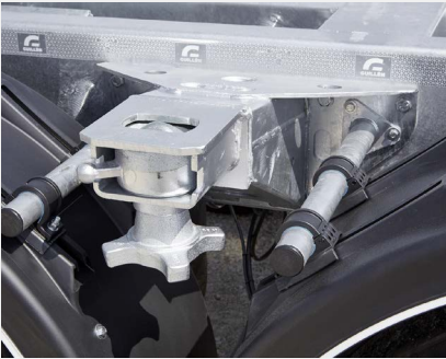
Bolt-on bolster for 20' container transport in central position
