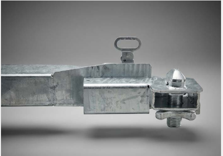
Removable twist lock on front extension for lower securing of non-High Cube containers (without tunnel)
