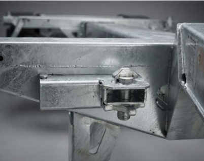
Removable twist lock on front extension for lower securing of non-High Cube containers (without tunnel)
