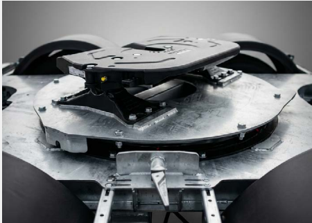
Fifth wheel mounted on a low-maintenance slewing ring, with manual locking for manoeuvring operations.
