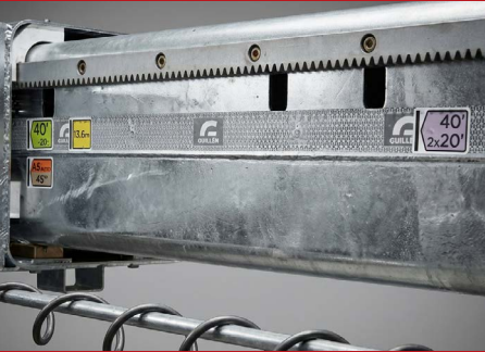
Rear extension system operated by a rack-and-pinion mechanism.
