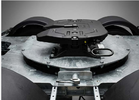
Fifth wheel mounted on a low-maintenance slewing ring, with manual locking disabled during manoeuvring operations.
