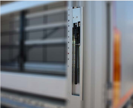
Hydraulic roof lifting system.
